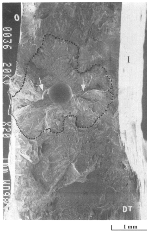
Fig. 21 SEM micrographs of cracked pore fracture surfaces. (a) Pore diameter, 0.015 in. (0.38 mm). Unheat-tinted fracture. Zone 1 boundary outlined for clarity. 13 \times . (b) Pore diameter, 0.025 in. (0.64 mm). Heat-tinted fracture (not evident in SEM). Zone 1 boundaries outlined for clarity. 20 \times .
