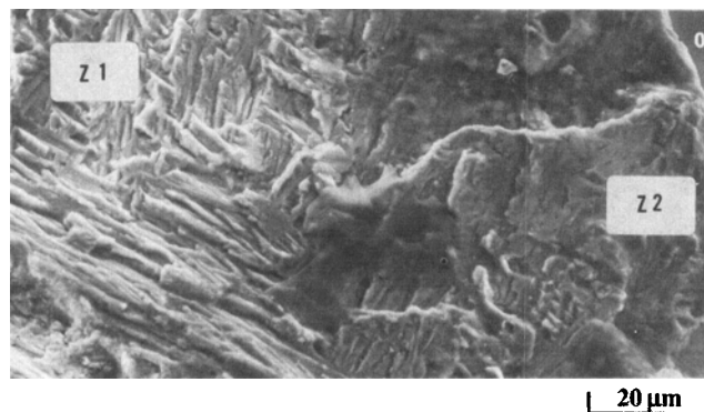
Fig. 12 The transition of Fig. 11 at higher magnification. 550 \times .
