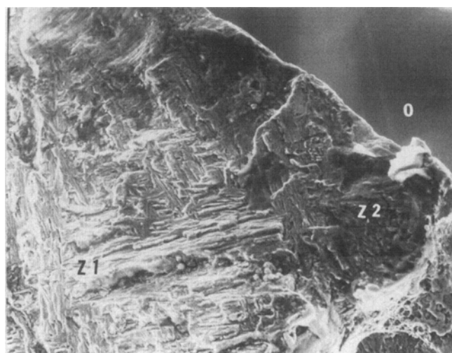
Fig. 11 Zone 1 to zone 2 transition near the outside vessel surface. 266 \times .
